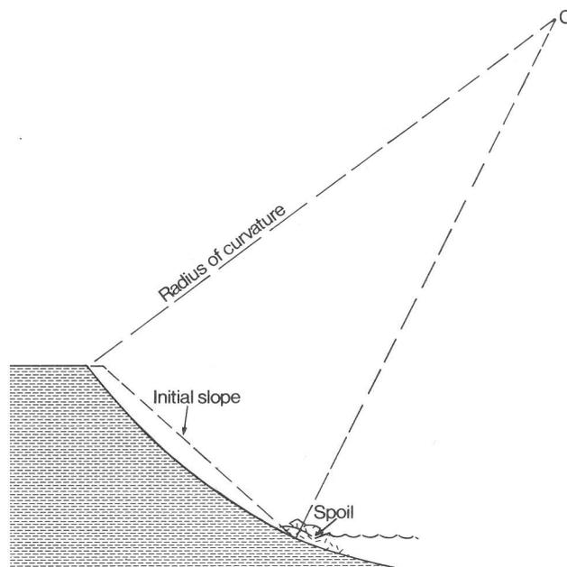
Figure 2a—Cross section of a sheet slide.
