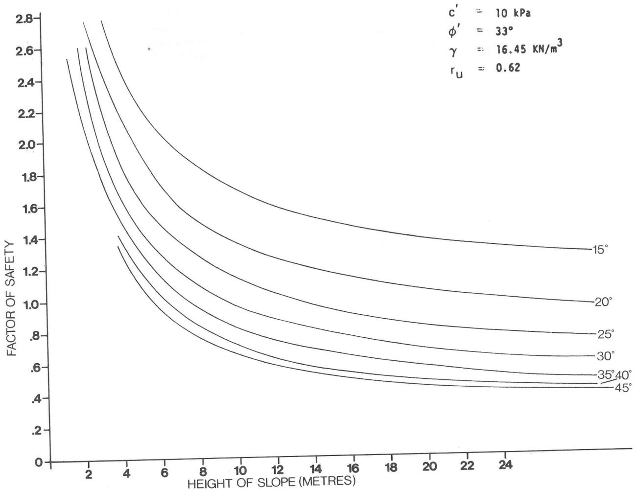
**Figure 5**—Diagram showing the relationships between the slope inclinations, the slope heights, and the Factors of Safety as computed for a study in the Ottawa area (Klugman and Chung 1976).
