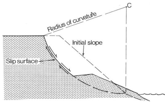
**Figure 2b**—Cross section of a simple rotational shear.
