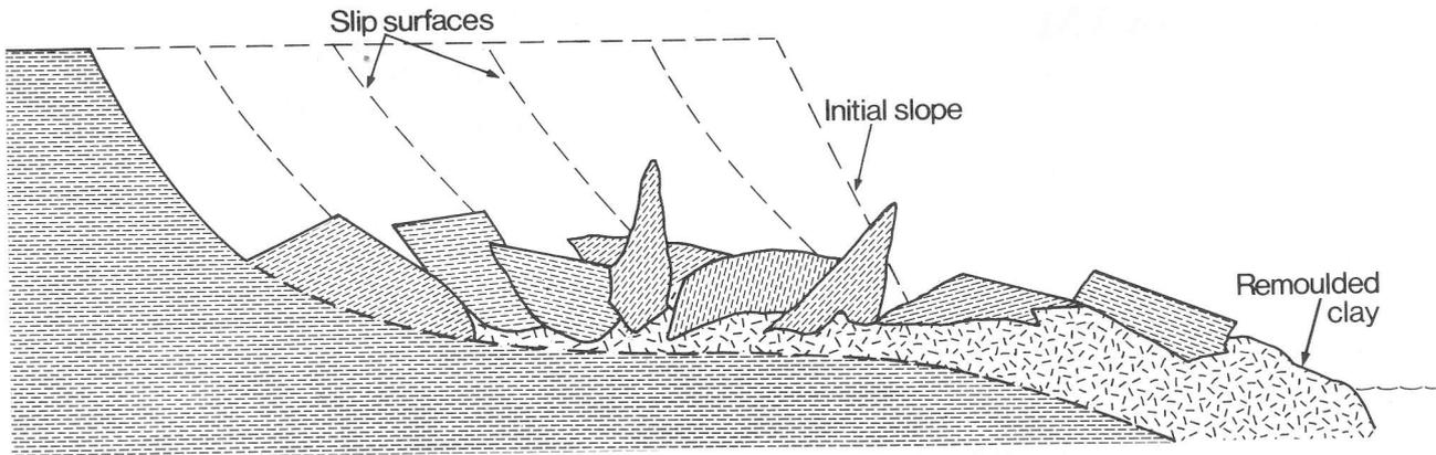
**Figure 3b**—Cross section of a retrogressive flowslide.
