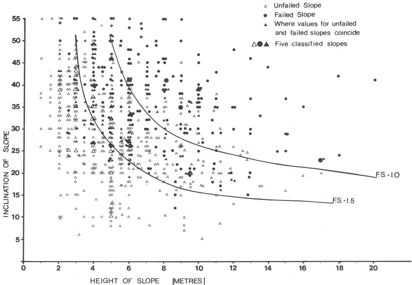
**Figure 6**—Diagram showing the relationships of failed and unfailed slopes in the study area to height, inclination, and the Factors of Safety of 1.0 and 1.5.
