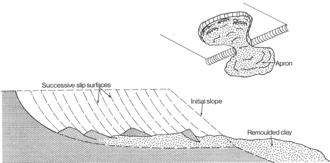
**Figure 4**—Cross section of an earth flow.
