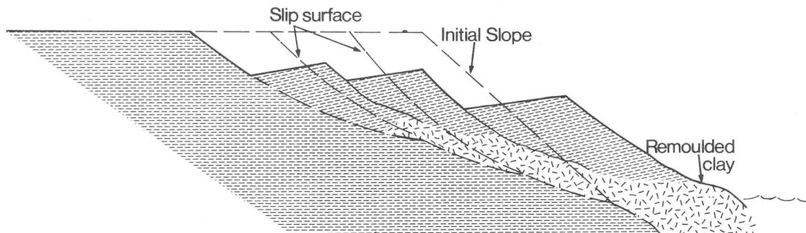
**Figure 3a**— Cross section of a retrogressive rotational shear.
