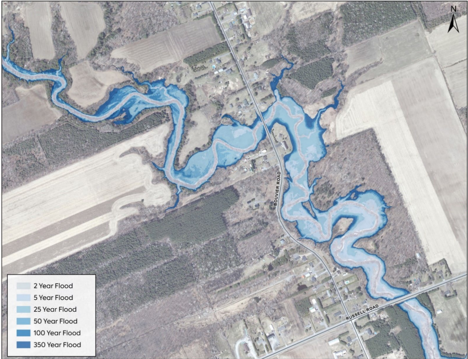
Figure 3. An example of flood extents with different annual exceedance probabilities in North Indian Creek generated through the Bear Brook Floodplain Mapping Project (SNC, 2024).
