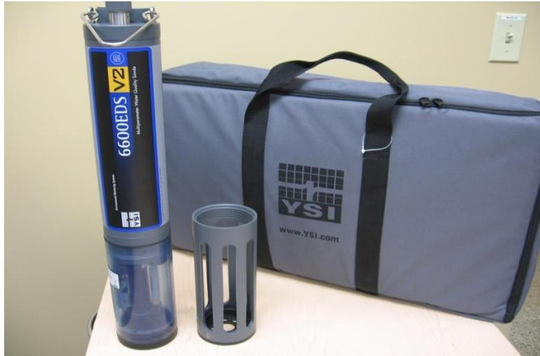
Photo 5. Equipment used for deployment of YSI Multi-parameter Water Quality Sonde Unit
