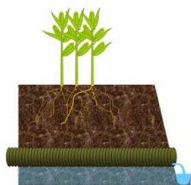
Figure 1: drainage non contrôlé
