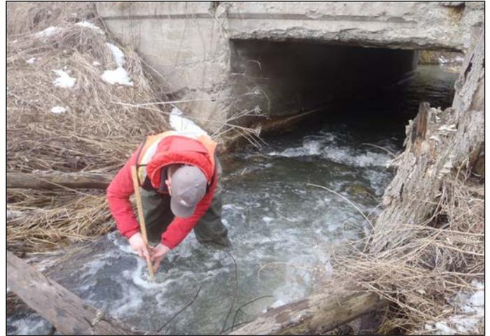
Volunteer measuring hydraulic head, a measurement of velocity, in a headwater drainage feature during spring freshet (period of snow melt)
