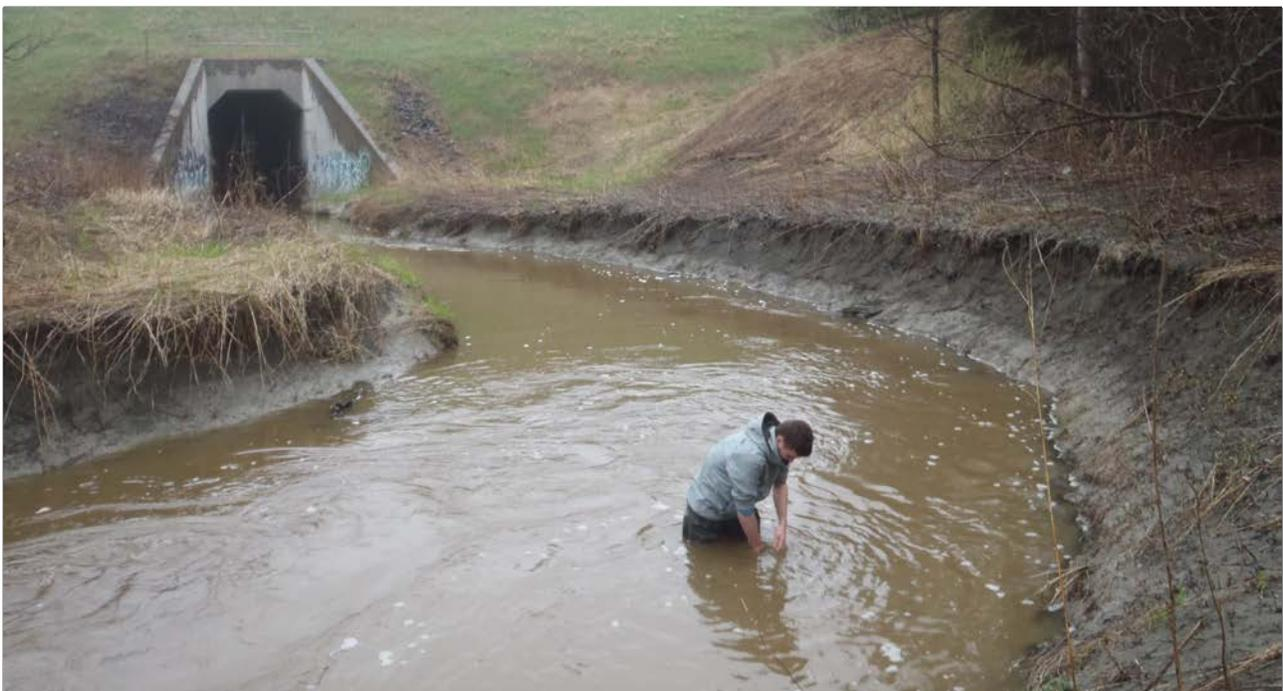
An RVCA summer student installing a temperature logger in Mud Creek in April
