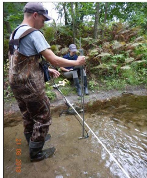
SNC staff taking baseflow measurements with highly accurate scientific equipment
