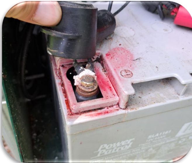
Corroded terminal due to bad battery
