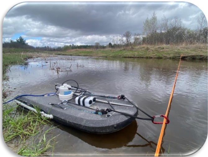
Flow measurements being taken at Hall Road monitoring site City of Ottawa
