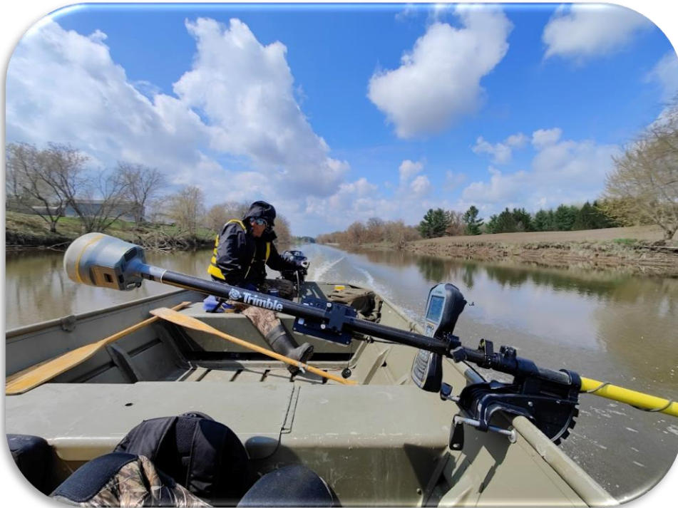
Staff conducting bathymetric survey on the Castor River
