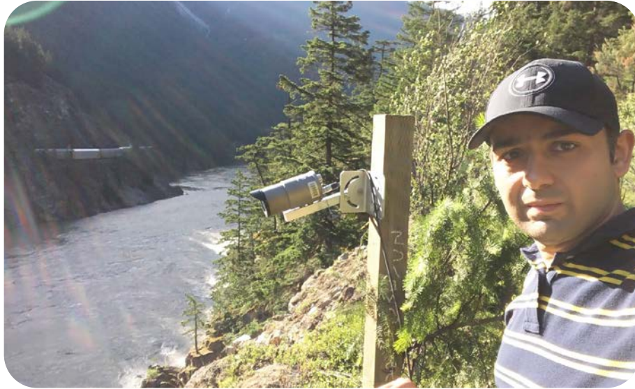
Installation of cameras to study river hydrodynamics Black Canyon, Fraser River, BC.
