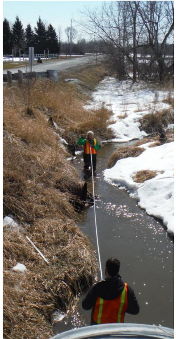
Measuring slope in the Mosquito Creek catchment
