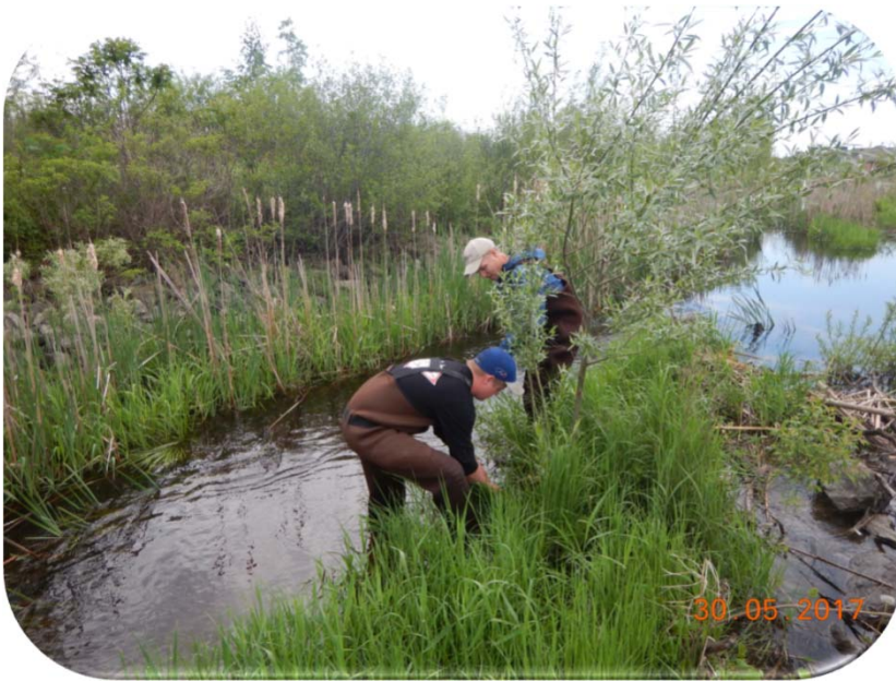
Staff deploying sensors in Findlay Creek
