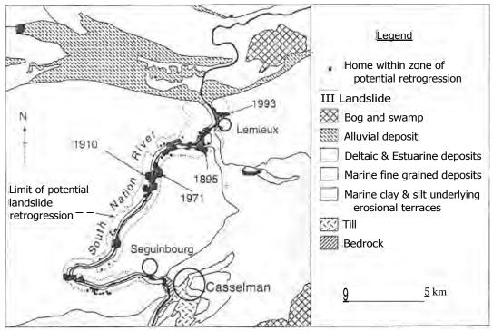
Figure 2. Study area along South Nation River, Casselman to Lemieux, showing surficial geology (after Richard, 1982), dates of landslides if known, limit of potential landslide retrogression and homes located within area of potential retrogression (Golder Associates, 1993).
