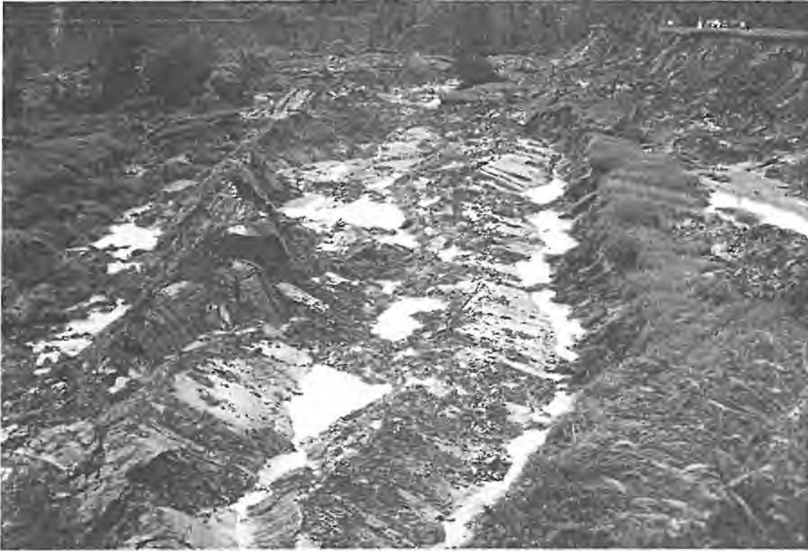
FIG. 6. The Lemieux landslide crater on June 21, 1993, about 24 h after the landslide took place. View is to the east along the south rim where onlookers (top right) provide scale. Note (from right to left) rotational blocks below the scarp, an exposed sliding surface within displaced blocks which formed along rotated lamination surfaces, clay ridges about 3 m in height, and sod from former field surface, and another clay ridge. Laminations in the clay ridges are horizontal.
