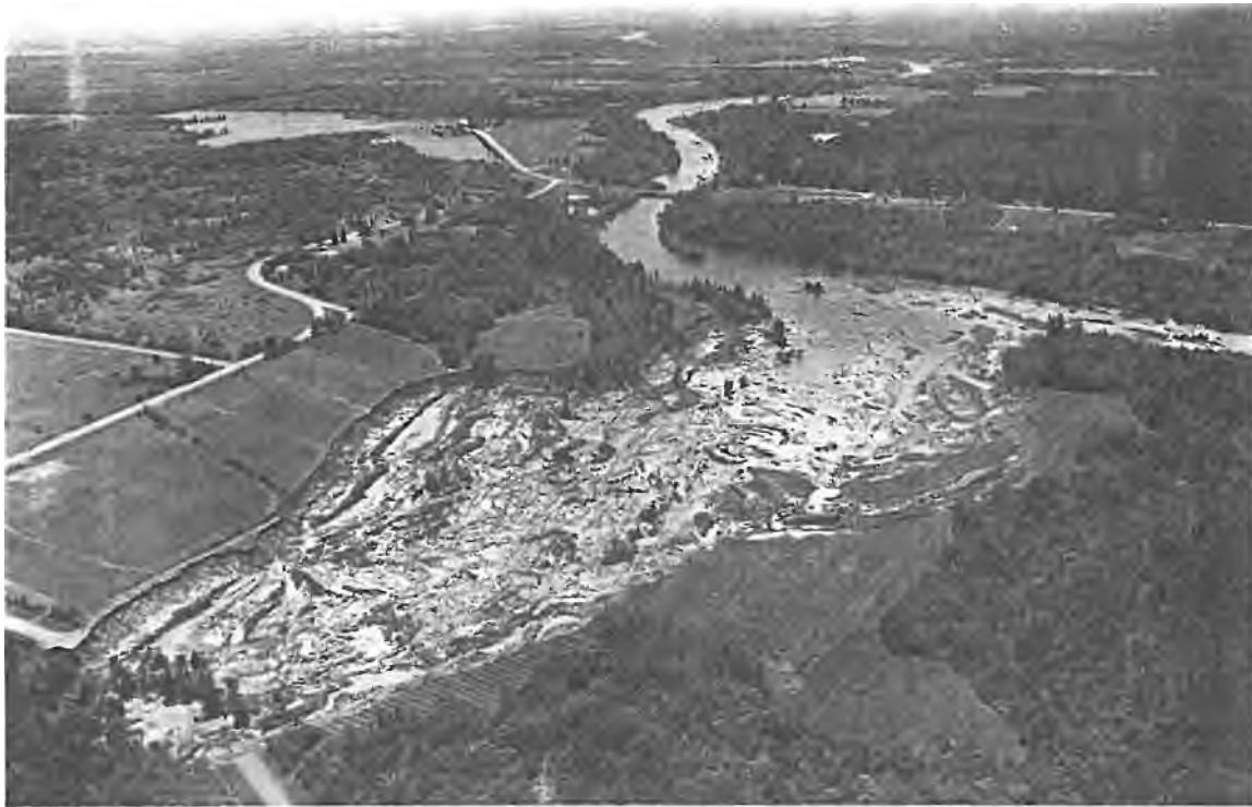
FIG. 1. Aerial view of the 1993 Lemieux landslide which took place on June 20, 1993. View is toward the southwest looking up the South Nation River. Severed County Road 16 is seen at bottom left and County Road 8 bridge discussed in text is seen upstream of the landslide in the middle distance. Note impoundment of river and upstream flooding. Photo taken on June 23, 1993.
