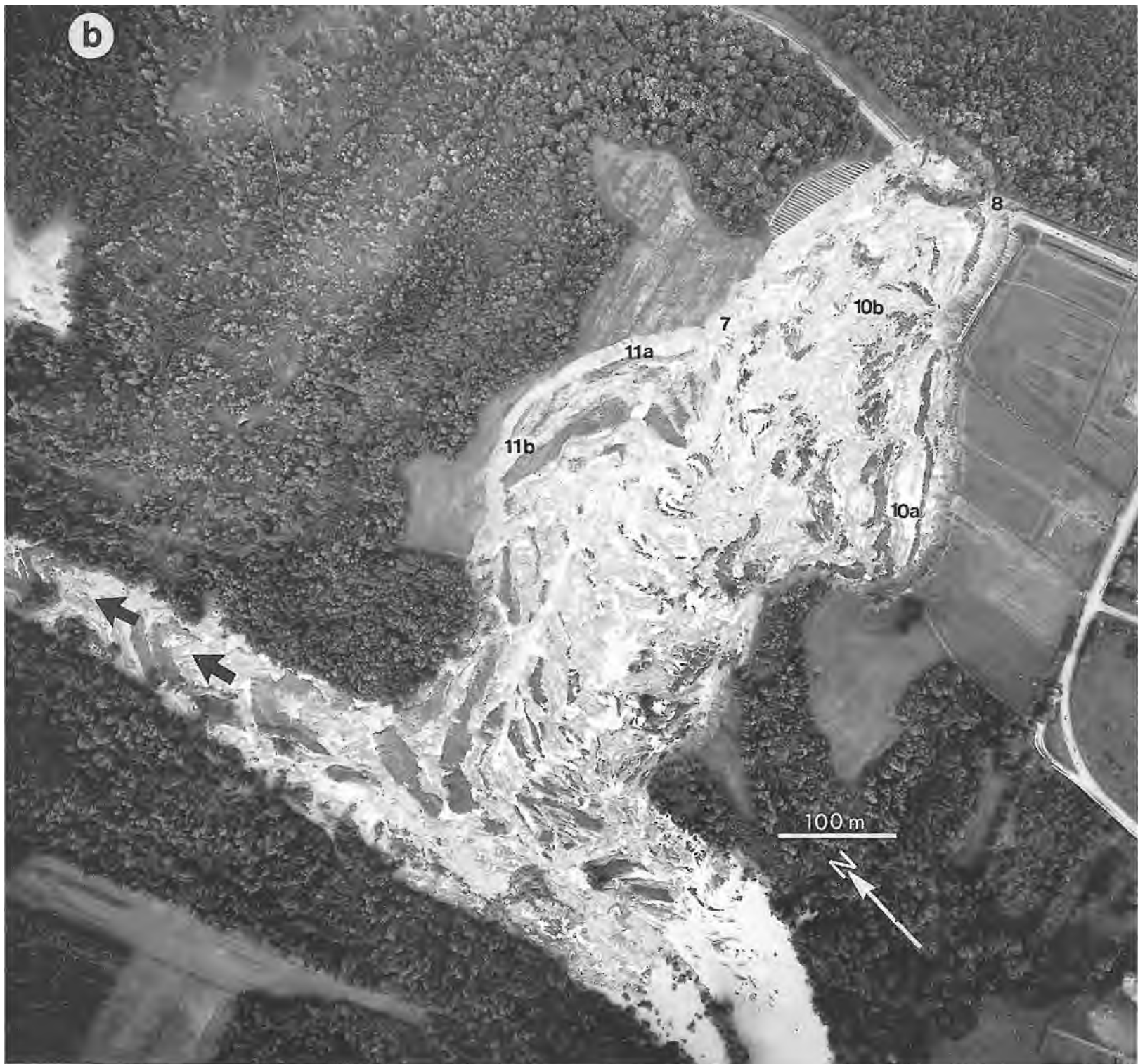
Photo b) was taken two days after the landslide and before the impounded river had overtopped the spoil in South Nation Valley. The landslide crater is 680 m long and up to 320 m wide, covering 17 ha (Evans and Brooks, in press). The elongated shape is not symmetrical; outward embayments extend from both its north and south side. Numbers refer to location of Figures 7, 8, 10a, 10b, 11a, 11b.
