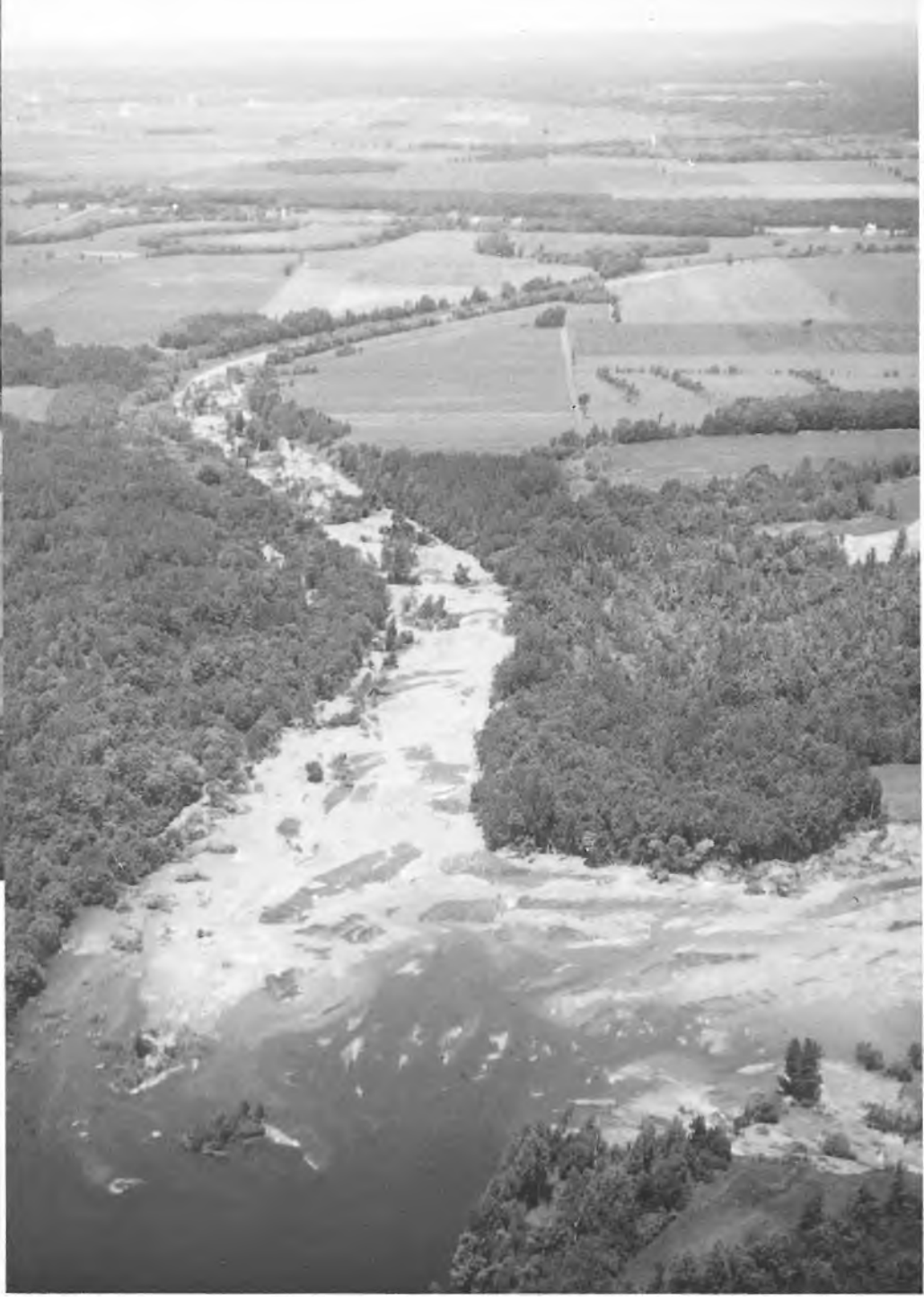
Figure 5. View downstream across the crater mouth showing the landslide spoil which travelled downstream along the valley bottom (GSC 1993-254A). It was taken late morning Wednesday, June 23, 1993, hours after the impounded river waters overtopped the landslide dam and began flowing downstream. Reflecting a rapid change in water turbidity, water colour changes from dark to light beginning at the mouth of the crater where flow starts to accelerate across the crest of the landslide dam causing erosion and entrainment of the spoil. High levels of water turbidity adversely affected water quality to farms and communities downstream for several days after the river flow was restored.
